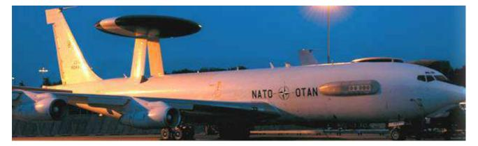
The NE-3A is a modified Boeing 707 equipped with long-range radar and passive sensors capable of detecting air and surface contacts over large distances. Information collected by AWACS can be transmitted directly from the aircraft to other users on land, at sea or in the air.
