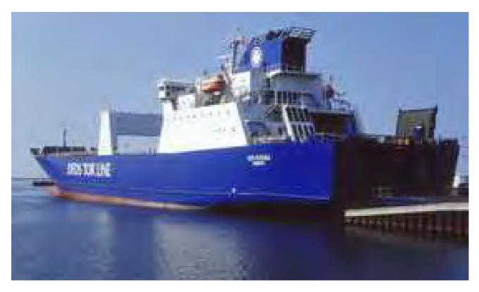
This multinational consortium finances the charter of up to 11 special "roll-on/roll-off" ships (commonly, Ro/Ro; so called because equipment can be driven onto and off of the ships via special doors and ramps into the hold). The consortium includes Belgium, Canada, Denmark, Germany, Hungary, Lithuania, the Netherlands, Norway, Portugal, Slovenia and the United Kingdom.
